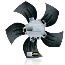
The condenser fans are designed for maintenance-free and low-noise operation. This is achieved through the use of deep groove ball bearings that are closed on both sides, along with specially paired grease lubricant. These features guarantee the reliable and quiet performance of the fans
