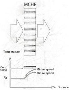
Increased efficiency with high and consistent Δt between refrigerant and ambient air
