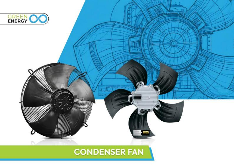
The direct-drive vertical discharge condenser fans are dynamically balanced to ensure smooth operation. These fans are equipped with totally enclosed air-over motors, which provide complete sealing of the motor windings to protect them from exposure to ambient conditions. The condenser fan motors are three-phase, featuring permanently lubricated ball bearings and internal thermal overload protection.
